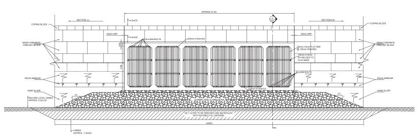
CULVERT GRATE ELEVATION-SEA SIDE VIEW
